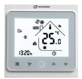
Voltage/ Frequency: 230 V AC / 50 - 60 Hz Maximum current: 5 A Operating temperature range: 0 - 45°C Regulation range: 5°C - 35°C Regulation accuracy: ± 0.5°C External temperature sensor: NTC 10K Communication: RS485 Dimensions: 86 × 86 × 13.3 mm Weight: 270 g Degree of protection (housing): IP 20 Degree of protection (external sensor): IP 68
