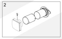
3 – Assemble the external pipe through the wall, so that the external inlet/outlet is on the outside of the building (3-1). Then turn the external pipe to place the inlet/outlet facing down (3-2 i 3-3) and pull it from the inner that the seal fits tightly to the facade (3-4).
