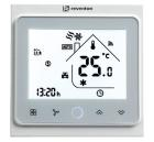
Voltage/ Frequency: 230 V AC / 50 - 60 Hz Maximum current: 5 A Operating temperature range: 0 - 45°C Regulation range: 5°C - 35°C Regulation accuracy: ± 0.5°C Communication: RS485 Dimensions: 86 × 86 × 13.3 mm 270 g Degree of protection (housing): IP 20
