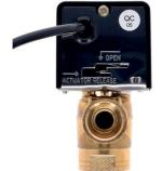
Power supply/ Frequency: 230 V AC/ 50 - 60 Hz Power consumption: 7 VA Kvs coefficient: 6.5 m³/h Operating condition of actuator: 0 - 60°C Running time (motor): 18 s Running time (return spring): 5 s Degree of protection: IP 20
